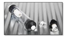
Pre-Filter Tubes – Glass tubes (also known as "scrubbing tubes" or "benzene tubes") that filter other gasses, leaving only benzene behind for detection by the PID sensor. Pre-Filter Tubes mount inside the tube holder and are sold in boxes of 10.
