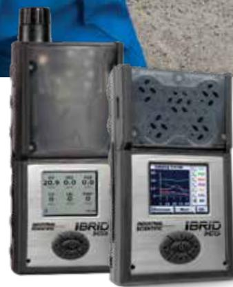
The MX6 iBrid® is more than an intelligent hybrid of Industrial Scientific's best monitoring technologies—it's the most adaptable six-gas monitor on the market. The MX6 iBrid uses five sensor slots to detect up to six gases. Each of those slots accepts a variety of sensors, which means you can use the instrument with a PID sensor one day and an infrared sensor the next. Settings allow you to adapt the instrument's behavior based on your application.
