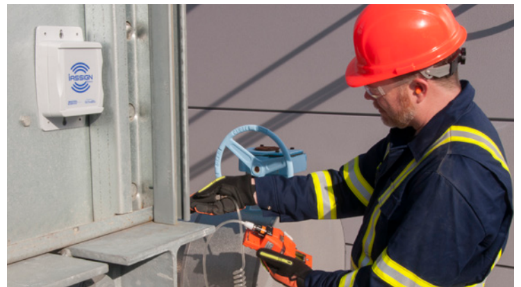
iAssign Beacons – Automatically assign location names to Ventis Pro Series Multi-Gas Monitors based on proximity, helping safety managers see where hazards occurred and who was involved.
