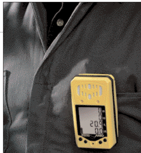
Atmospheric conditions within a confined space can change rapidly, making it very important to continuously monitor for gas hazards.
