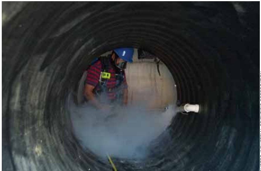
Top: A trainee gets hands-on experience in testing a confined space simulator's internal atmosphere prior to entry. Above: A confined space simulator adds theatrical smoke to show the trainee how gas stratifies within a space.
