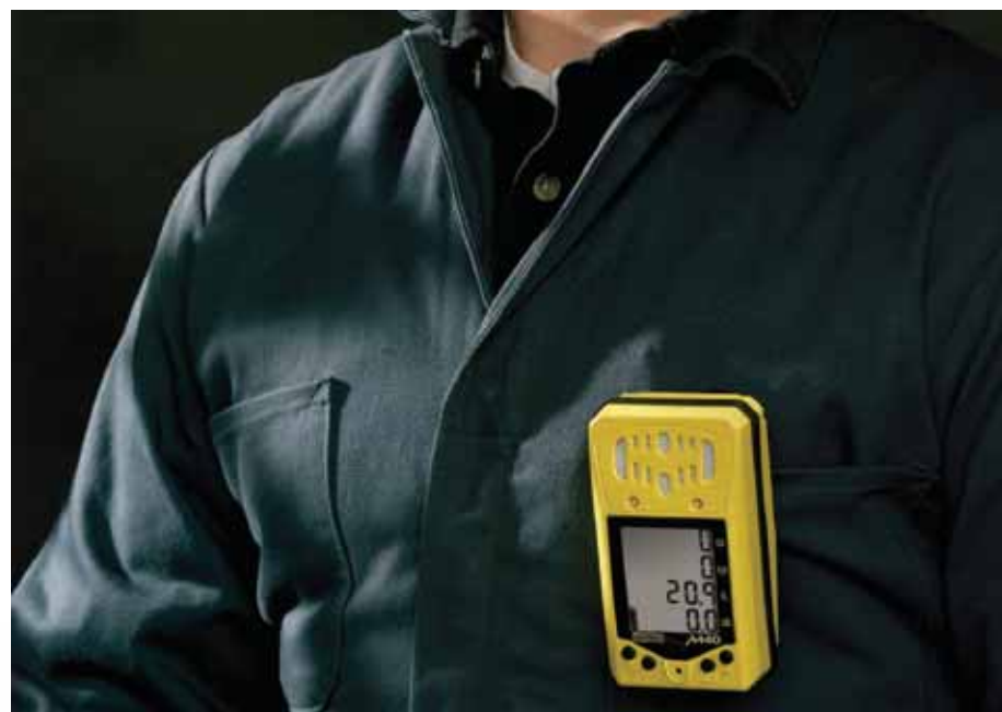
Figure 2: Compact sized, personal multi-gas monitors are ideal for a wide variety of hazardous and confined space applications.
