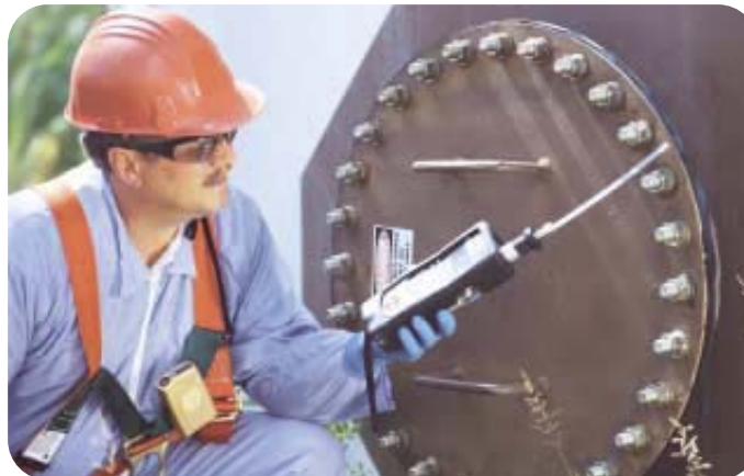
Photoionization detectors (PIDs) are gas monitors that levels of hydrocarbons down to sub-ppm levels.
